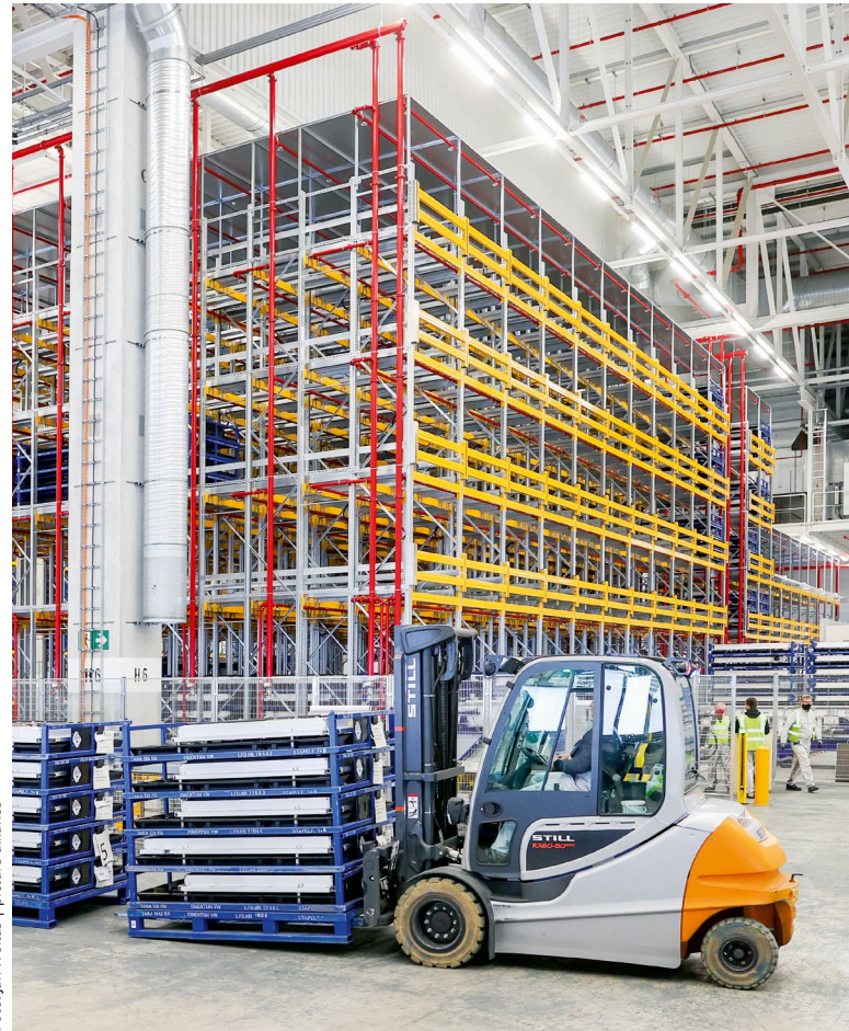
Batteries for electric vehicles produced on a large scale are stored and transported unpackaged in metal load carriers.
